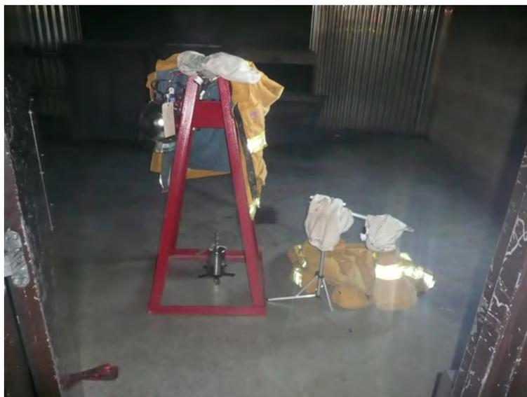
Figure 5. Area air sampling set-up for Exercise 5.
